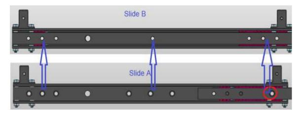
blocked by the inner slide, then you can use the hole marked by the red circle add screw.
