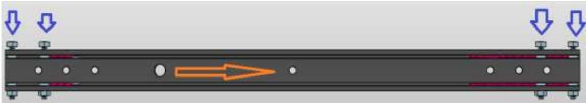
2. Attach the pulley module on the end of slide by letting the screws going through the holes of the pulley module. Put the nuts back to the screws.
